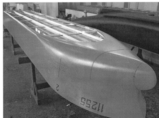
Figure 12 Model 01010 of a cargo ship with the recess for wavy cavity, interior keels and cavitators in Krylov Ship Research Institute.
